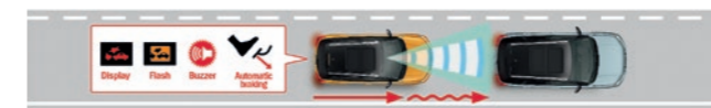
Applies strong automatic braking if the risk of collision increases even more
