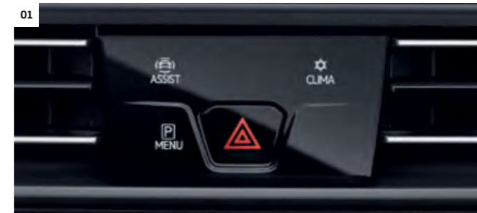
01 Direct access button module. The module is arranged centrally around the hazard warning lights button and uses shortcuts for easy access to major functions such as driver assistance systems, air conditioning functions and parking assistance systems. | C | L |
