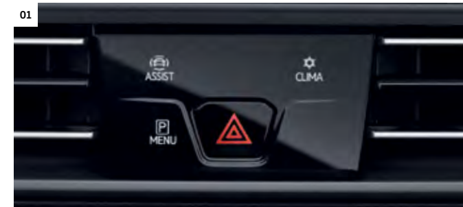
01 Direct access button module. The module is arranged centrally around the hazard warning lights button and uses shortcuts for easy access to major functions such as driver assistance systems, air conditioning functions and parking assistance systems*.
