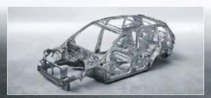
The SGP and ring-shaped passenger safety cell absorb and direct impact force around the cabin, rather than through it.
