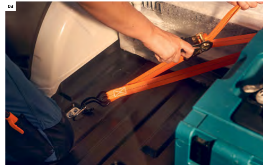
03 Lashing eyes. Keep their promise. The six folding lashing eyes secure heavy loads rock-solid on the vehicle floor of the Caddy Cargo. | C |
