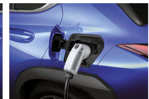
DC charging inlet
