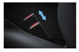
Easy Access Buckles (Front seats - Sports Luxury models)<sup>1</sup> To make the front seatbelts easy to use, the seatbelt buckle lifts
