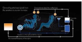
ANC (Active Noise Control) and Acceleration Sound Control (ASC) were fine-tuned to enhance the flagship-level quietness in the cabin, and at the same time enliven driving enjoyment. ANC suppresses engine boom at a wide range of engine speeds, while ESE tunes the sound of engine acceleration and deceleration to provide a powerful and linear sporty engine note.
