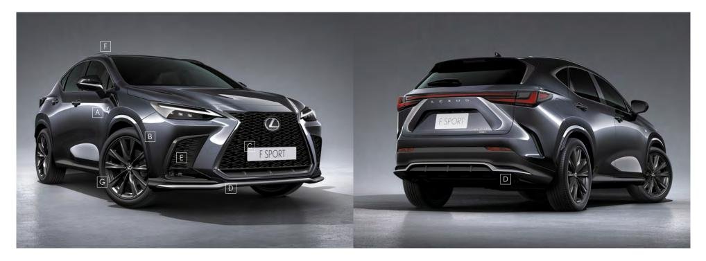
A\_F SPORT emblem / B\_Fender arch moldings / C\_Grille / D\_Lower bumper spoiler / E\_Garnish / F\_Roof rails (black) / G\_Exclusive 20-inch aluminium wheels
