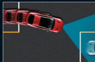
Autonomous Emergency Braking (AEB) 1 (with Junction Assist)
