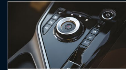
Shift-By-Wire Rotary Dial (HEV GT-Line & EV)
