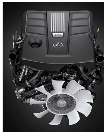
3.5-Litre V6 twin-turbo engine
