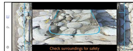
Back Underfloor View & Both-sides View
