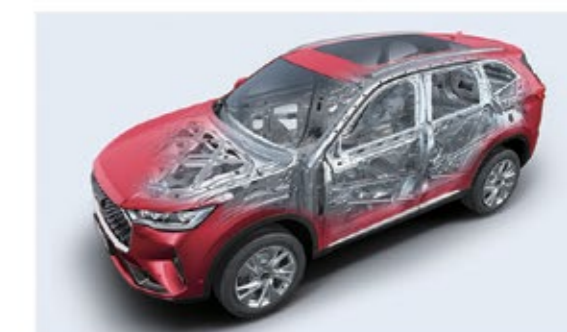
High-strength Steel Body
