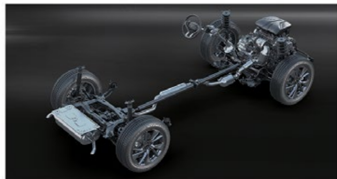
Front Macpherson Rear Multi-link Independent Suspension + AWD
